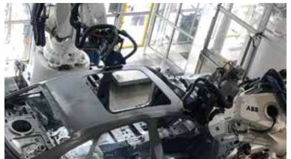
Jointly developed with ABB Specifically designed for laser weld grinding applications on car roofs
